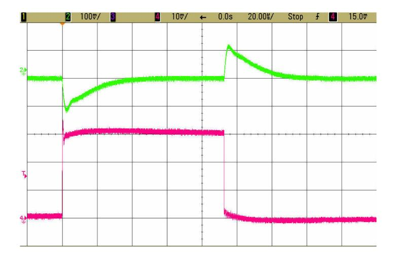
Figure 3.  $V_{OUT1}$  Load Step Response
