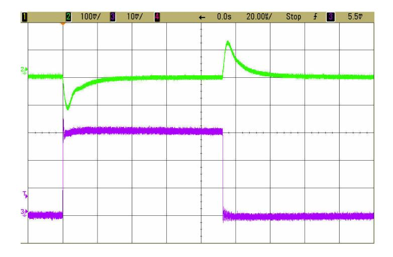
Figure 4.  $V_{OUT2}$  Load Step Response
