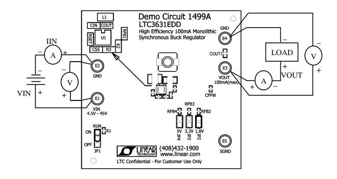
Figure 2. Equipment setup to test LTC3631
