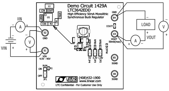
Figure 2. Equipment setup to test LTC3642
