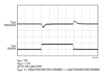
Figure 3. Measured Load Transient Response
