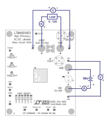
Figure 1. Test Setup of DC1414A
