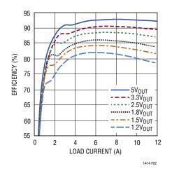
Figure 2. Measuring Supply Efficiency with Different  $V_{OUT} \left( V_{IN} = 12V \right)$
