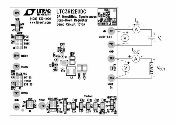
Figure 1. Proper Equipment Measurement Set-Up
