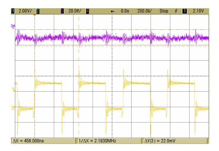
Figure 3. Switch Node & Output Ripple Voltage Waveforms  $V_{IN}$  = 3.3V,  $V_{OUT}$  = 1.8V,  $I_{OUT}$  = 3A
