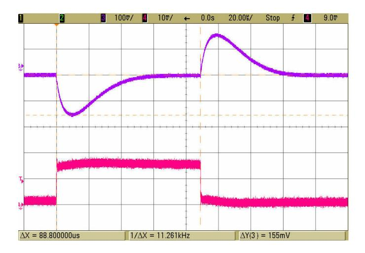
Figure 4. Load Step Response V<sub>IN</sub> = 3.3V, V<sub>OUT</sub> = 1.8V, 2.5A Load Step (0.5A <-> 3A) Forced Continuous Mode Fsw = 2 MHz
