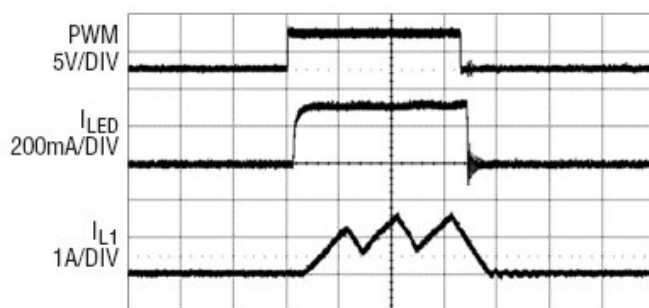
Figure 2. DC1279A 30V LED string PWM Dim, PVIN=12V
