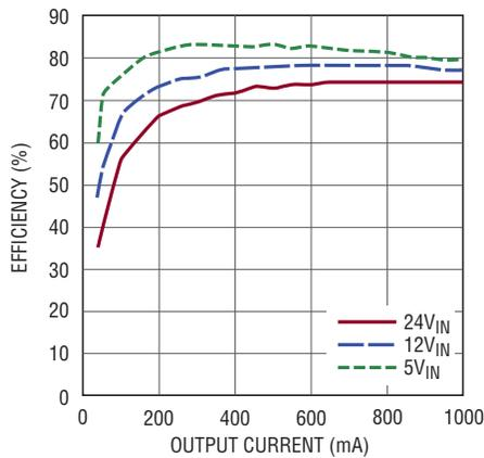
Figure 2. Efficiency with Single 3.3V<sub>F</sub> LED at 1A. LED Current is Adjusted with ADJ Voltage
