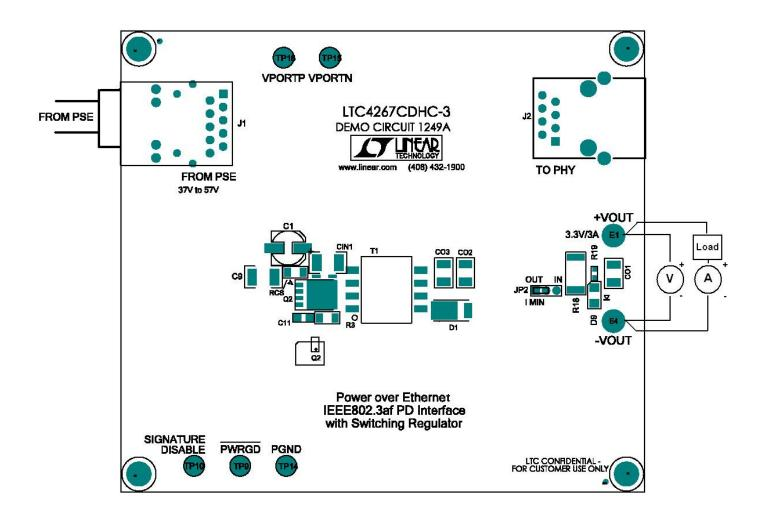
Figure 1. Proper Measurement Equipment Setup
