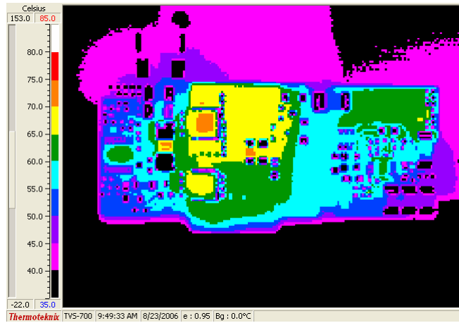
Figure 9. Temp Data (36Vin, 20A, 25°C, 200LFM airflow – back)
