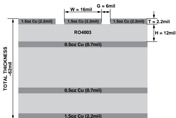
Figure 40. Probe Matrix Board Stackup, Cross Sectional View
