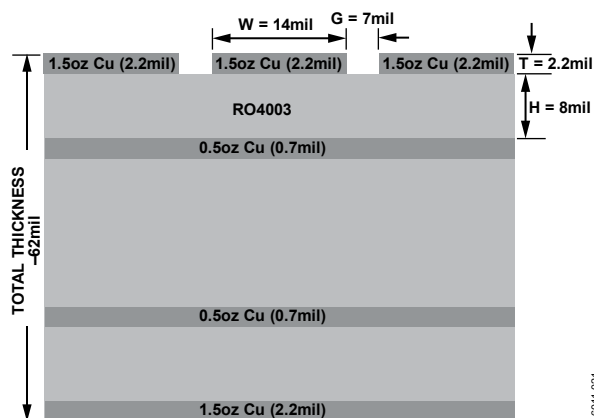
Figure 22. Probe Matrix Board (Cross Section View)
