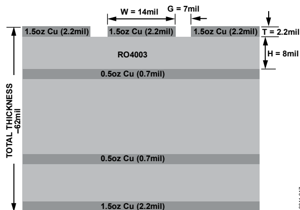
Figure 17. Evaluation Board (Cross Section View)
