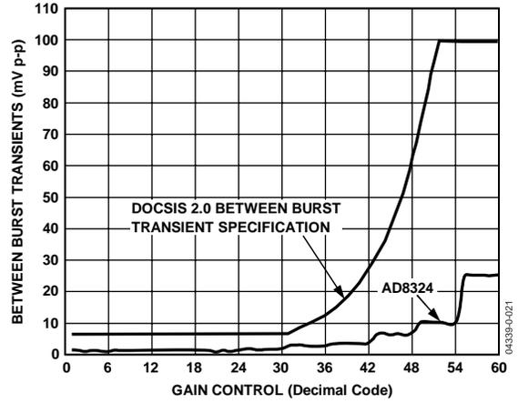
Figure 21. Between Burst Transient vs. Gain Control
