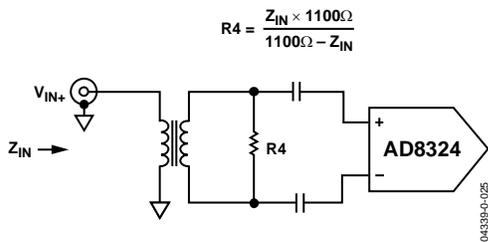
Figure 25. Single-to-Differential Circuit
