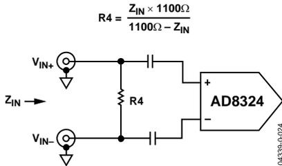
Figure 24. Differential Circuit
