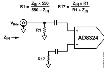
Figure 26. Single-Ended Circuit
