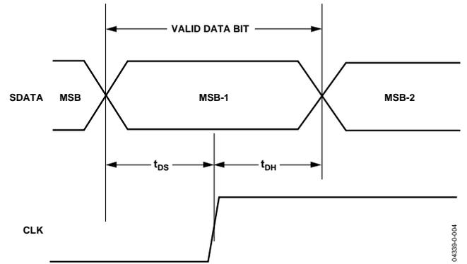
Figure 4.  $\overline{SDATA}$  Timing
