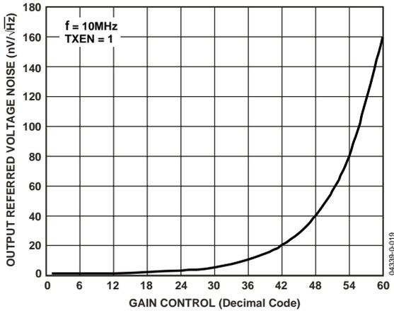
Figure 19. Output Referred Voltage Noise vs. Gain Control
