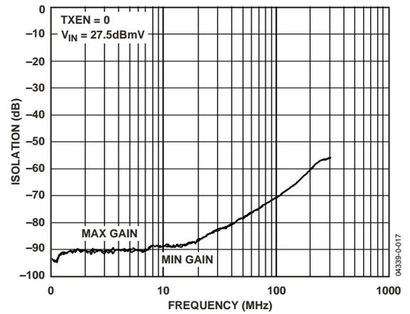
Figure 17. Isolation in Transmit Disable Mode vs. Frequency
