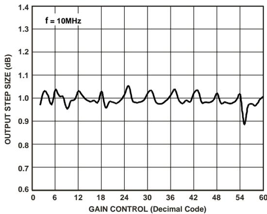
Figure 15. Output Step Size vs. Gain Control
