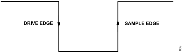
Figure 65. SPI Mode 3, SCLK Edges
