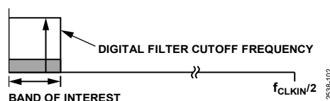
Figure 85. \Sigma - \Delta ADC Operation, Removal of Noise Energy from the Band of Interest (Linear Scale X-Axis)
