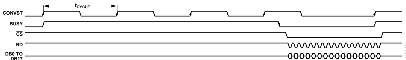
Figure 90. External Oversampling Clock Applied on the CONVST Pin (OSR = 4), Parallel Interface
