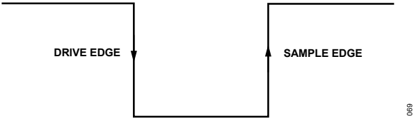
Figure 65. SPI Mode 3, SCLK Edges
