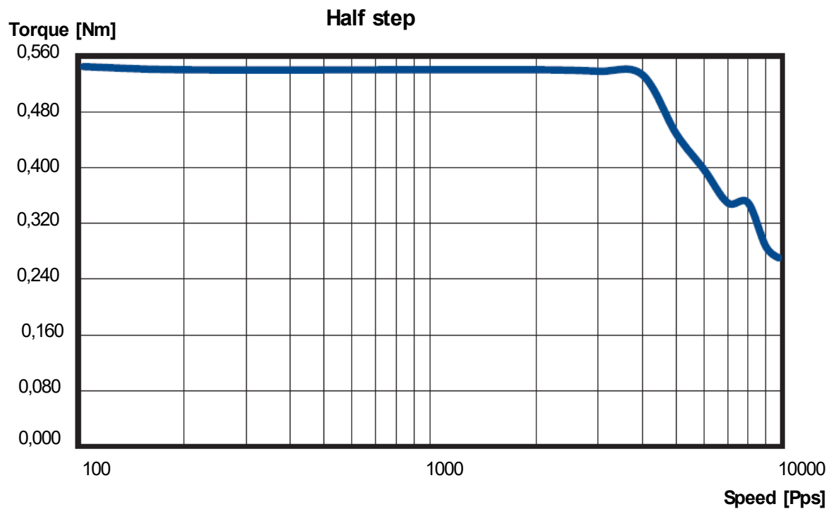
Figure 5.1: QSH5718-41-28-055 speed vs. torque characteristics
