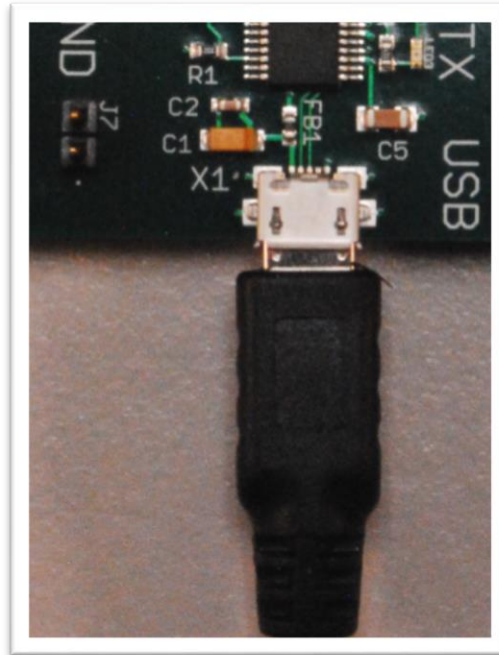
Figure 4 – USB Cable Connection
