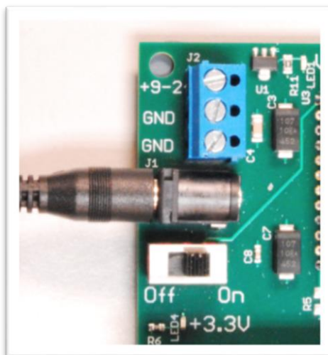
Figure 7 – Power ON Switch location
