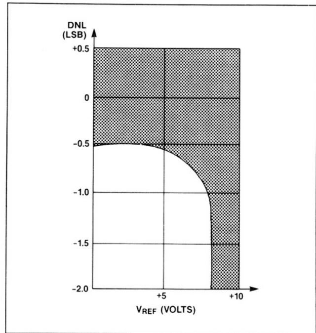
Figure 7. Differential Nonlinearity vs. Reference Voltage for Figure 4 Circuit.  $V_{DD}$  = 15 Volts. Shaded Area Shows Range of Values of Differential Nonlinearity that Typically Occur for L, C, and U Grades.
