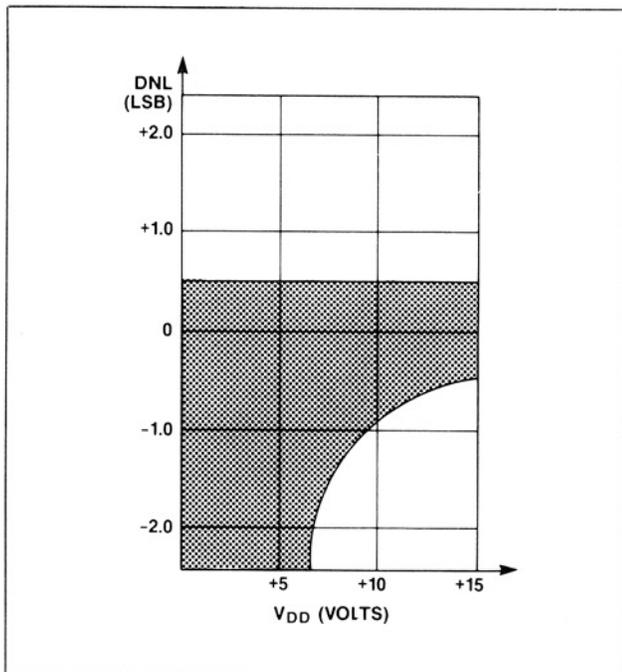
Figure 6. Differential Nonlinearity vs.  $V_{DD}$  for Figure 4 Circuit. Reference Voltage = 2.5 Volts. Shaded Area Shows Range of Values of Differential Nonlinearity that Typically Occur for L, C and U Grades.
