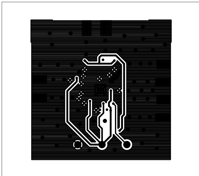
Figure 7. MAX9994 EV Kit PC Board Layout—Inner Layer 3 (Routes)
