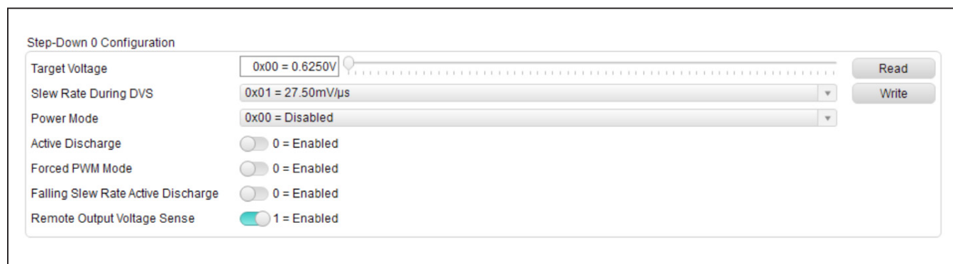
Figure 4. Step Down Configuration Portion of the EV Kit GUI
