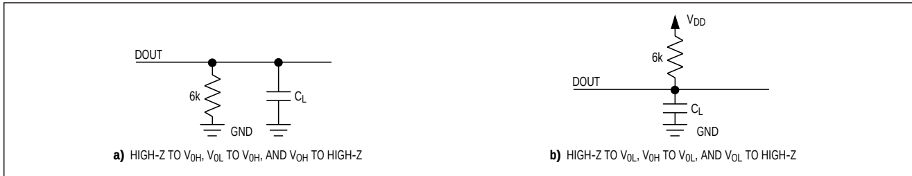
Figure 1. Load Circuits for Enable and Disable Time
