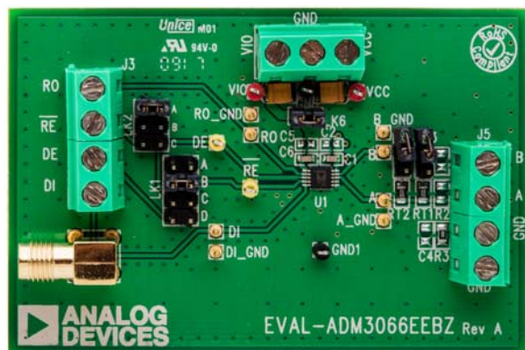
Figure 1. EVAL-ADM3066EEBZ Evaluation Board
