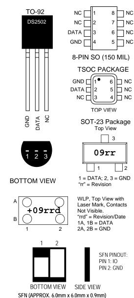
NOTE: THE SFN PACKAGE IS QUALIFIED FOR ELECTRO-MECHANICAL CONTACT APPLICATIONS ONLY, NOT FOR SOLDERING. FOR MORE INFORMATION, REFER TO APPLICATION NOTE 4132: ATTACHMENT METHODS FOR THE ELECTRO-MECHANICAL SFN PACKAGE.
