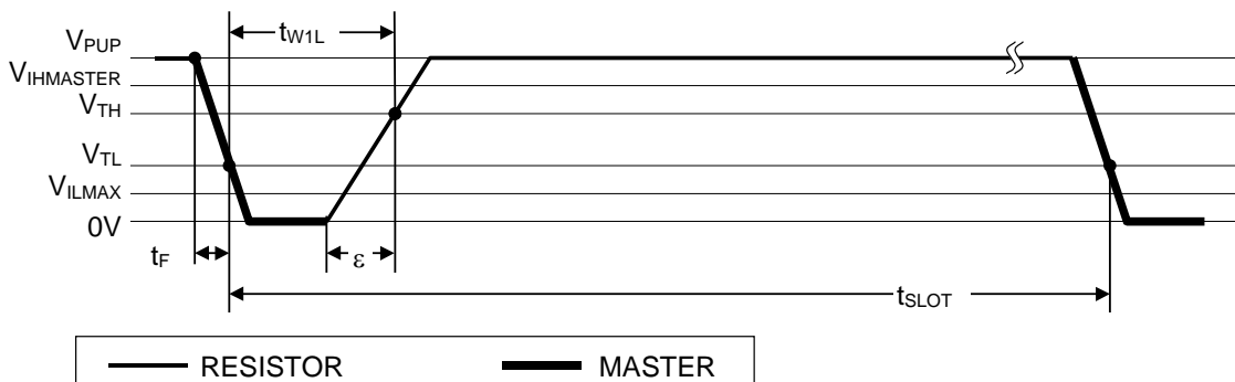
Figure 11. READ/WRITE TIMING DIAGRAM
