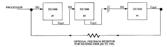
The  $C_{OUT}$  output of the DS1868B can be used to drive the DQ input of another DS1868B. When connecting multiple devices, the total number of bits transmitted is always 17 times the number of DS1868Bs in the daisy chain.
