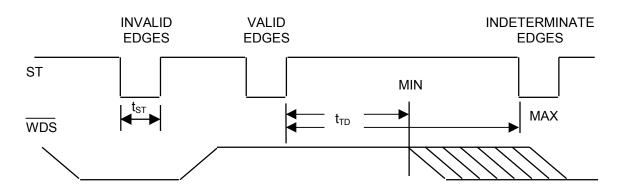
RESET TIMING DIAGRAM—POWER UP Figure 12
