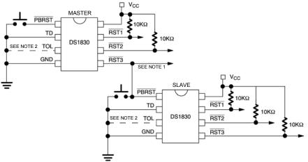
**Note 1:** The  $\overline{RST3}$  output tied to the pushbutton reset would be pulled to  $V_{CC}$  through the 40k $\Omega$  resistor in the pushbutton input. If a stronger pull-up is required an additional pull-up resistor could be added.
