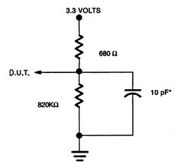
\* INCLUDING SCOPE AND JIG CAPACITANCE
