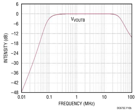
Figure 10. LT1568 Fourth Order Highpass Filter
