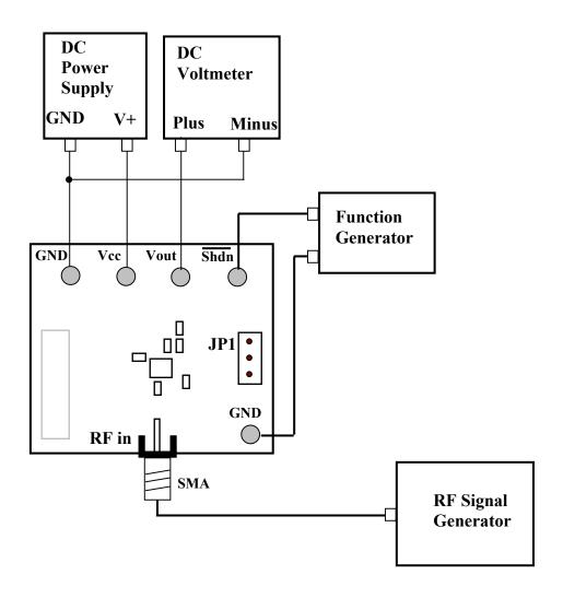
DC539A Demo Board Connection Diagram
