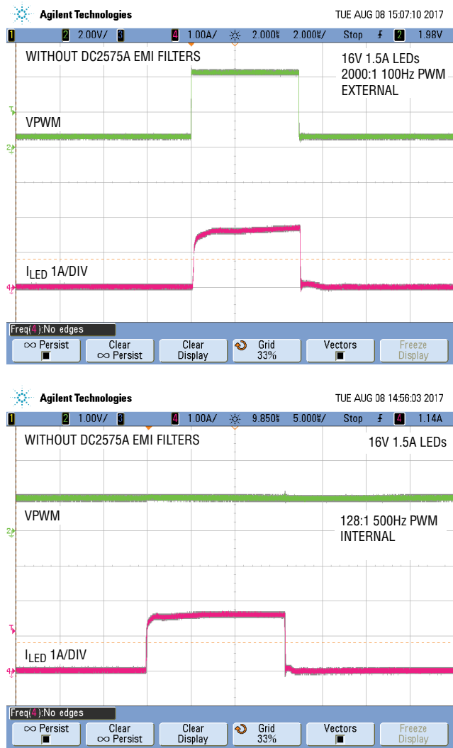
Figure 4. Infinite-Persist Scope Traces Show PWM Dimming and SSFM Working Together for Flicker-Free Brightness Control with Both (a) Externally- and (b) Internally-Generated PWM Dimming (with EMI Filters Removed)
