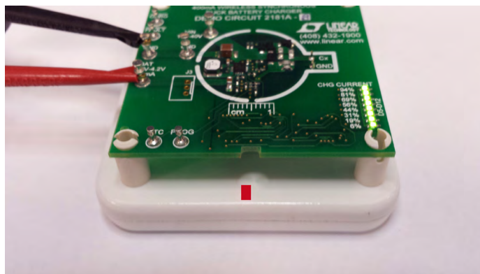
Figure 5c. DC2181A-A/B Wireless Power Demo Board Mounted on PowerByProxi's ProxiPoint Transmitter
