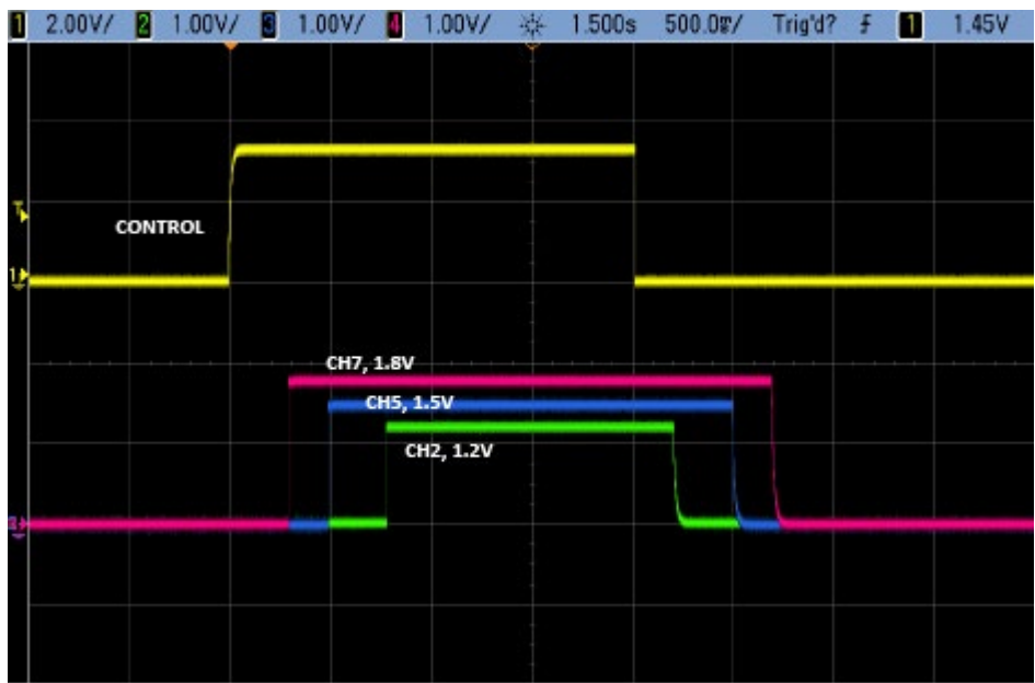
Figure 6. Sequencing Output Channels with DC2023A Using TON_DELAY and TOFF_DELAY
