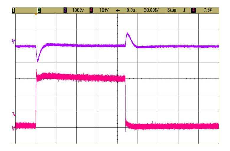
Figure 3.  $V_{OUT1}$  Load Step Response
