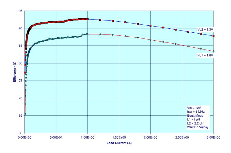
Figure 5. LTC3633 DC1347 Efficiency
