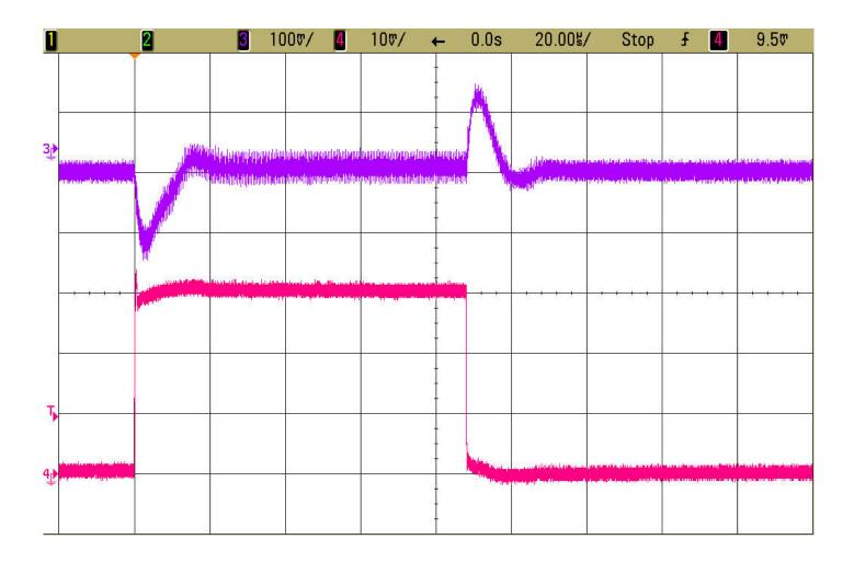
Figure 4.  $V_{OUT2}$  Load Step Response
