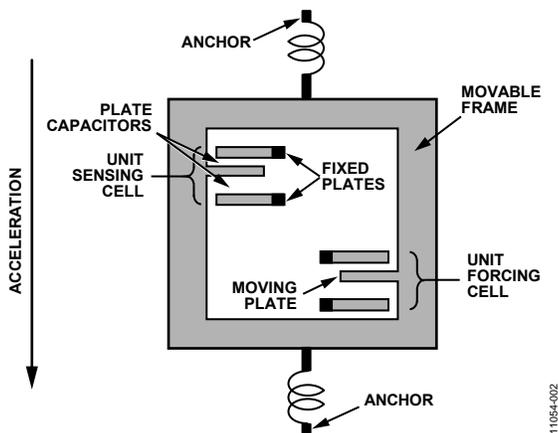
Figure 2. Simplified View of Sensor Under Acceleration
