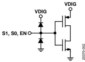
Figure 3. S1, S0, and EN Interface Schematic (Input)
