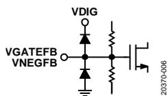
Figure 7. VGATEFB, VNEGFB Interface Schematic (Input)
