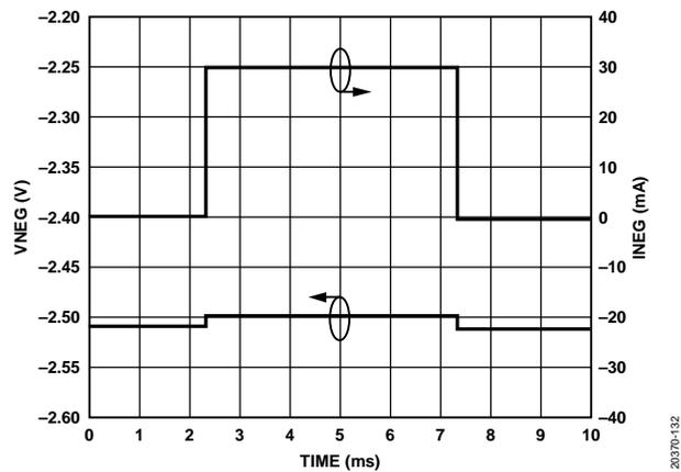
Figure 32. VNEG Load Transient, VDD = 16.5 V
