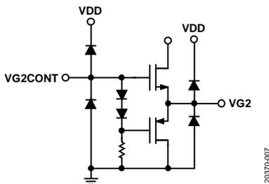
Figure 8. VG2 (Output) and VG2\_CONT (Input) Interface Schematic
