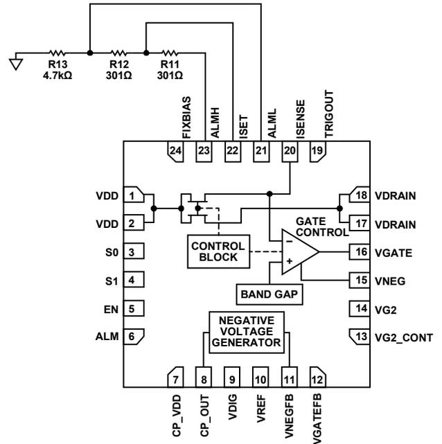
Figure 37. Current Alarm Resistor Configuration for ±6% Thresholds
