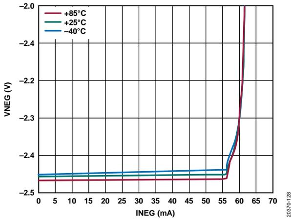
Figure 28. VNEG Load Regulation at VDD = 16.5 V
