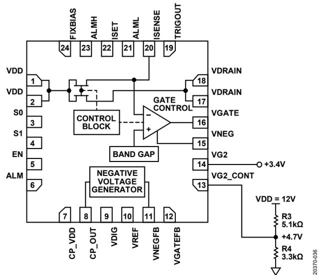
Figure 36. Resistor Divider Used to Set VG2
