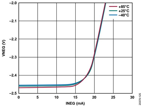
Figure 27. VNEG Load Regulation at VDD = 5 V
