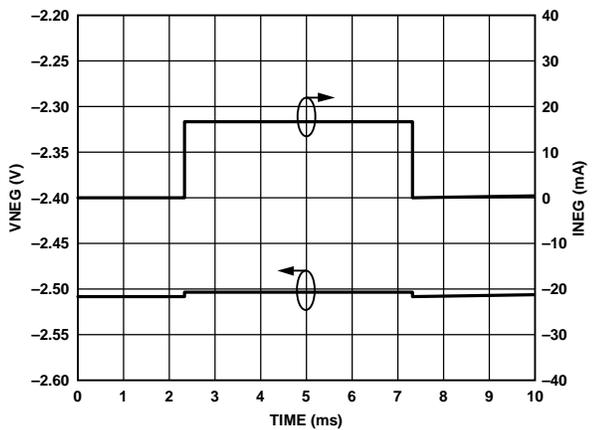
Figure 29. VNEG Load Transient, VDD = 5 V
