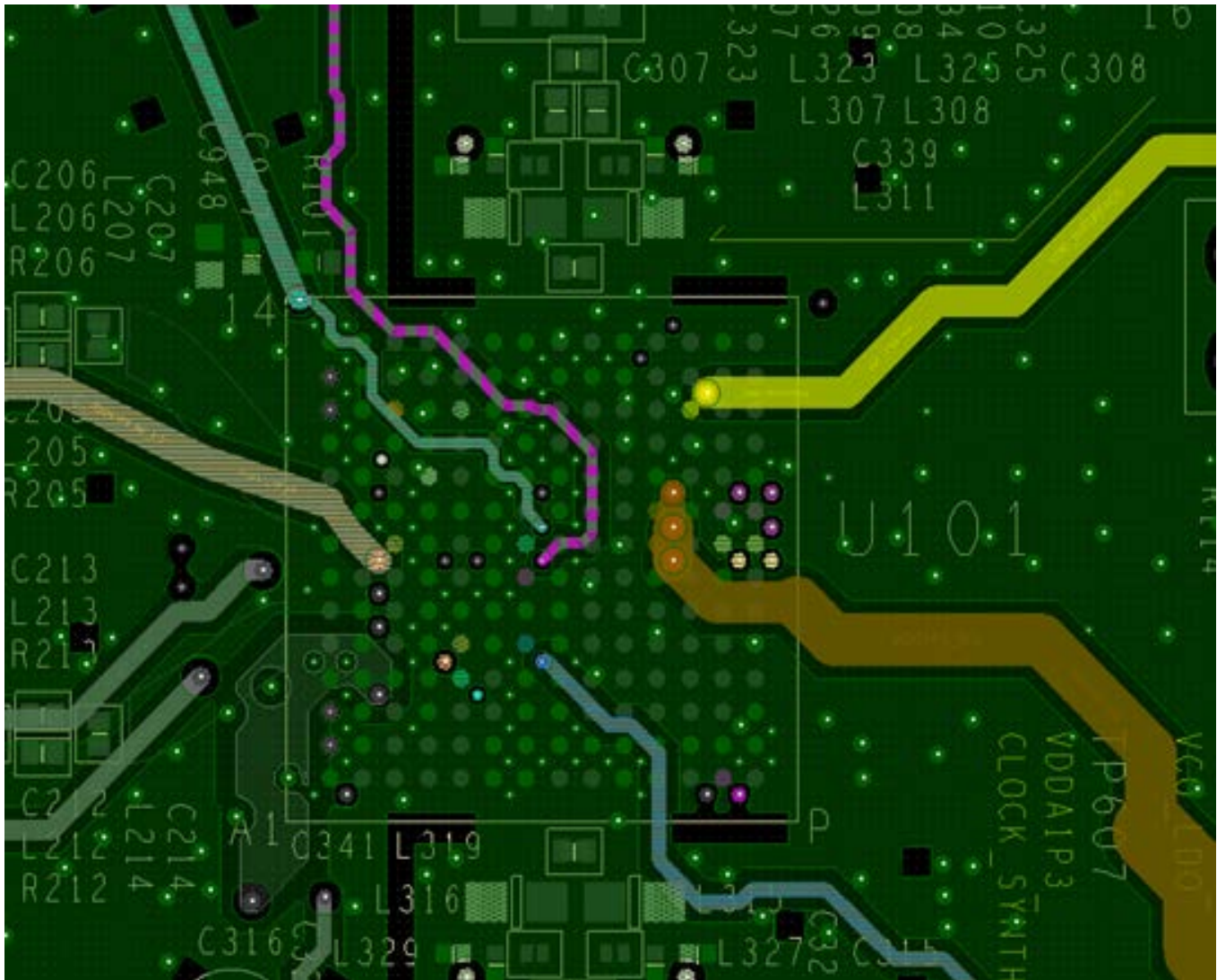
Figure 273. Layout Example of Power Supply Domains Routd with Ground Shielding (Layer 12 to Power)
