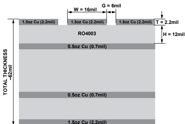
Figure 41. Probe Matrix Board Stackup
