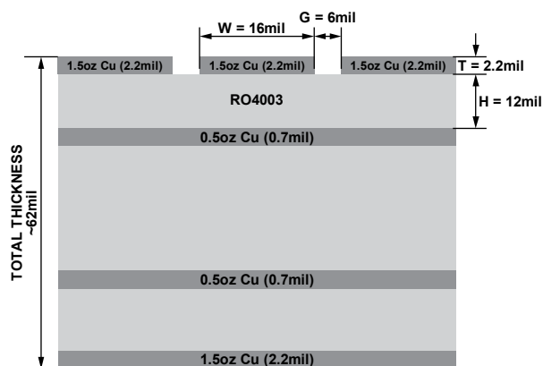
Figure 31. Probe Matrix Board (Cross Sectional View)
