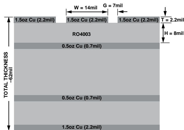
Figure 17. Probe Matrix Board Stack Up
