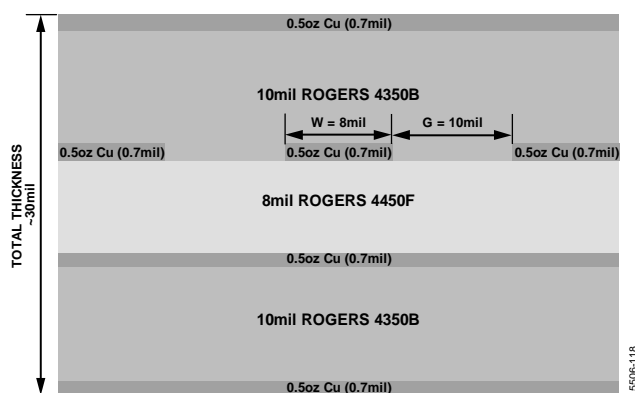
Figure 19. Evaluation Board Cross Sectional View
