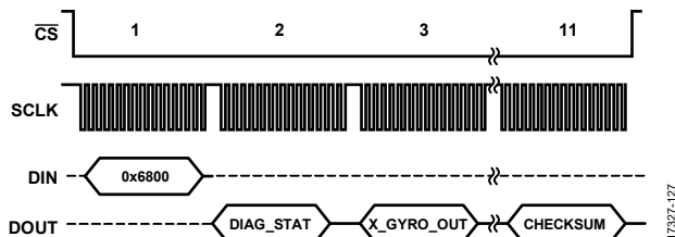
Figure 35. Burst Read Sequence with BURST_SEL = 0
