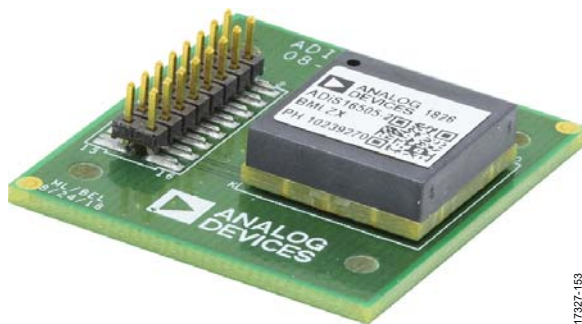
Figure 56. ADIS16500 Breakout Board ( ADIS16505-2 Shown)
