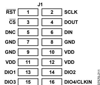
Figure 17. J1 Pin Assignments for the [ADIS16IMU2/PCBZ](#)
