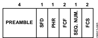
Figure 89. ACK Frame Format
