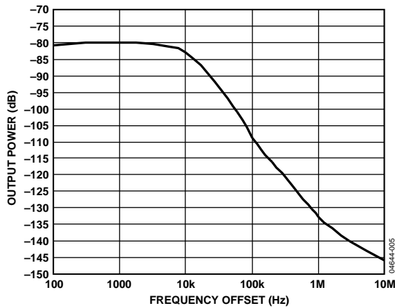
Figure 5. VCO Phase Noise, 2600 MHz, 200 kHz PFD, 10 kHz Loop Bandwidth
