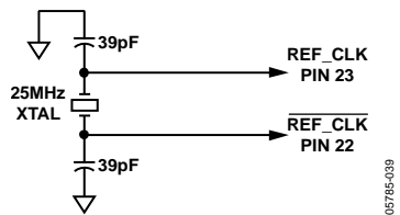
Figure 40. Crystal Configuration for Reference Clock Source
