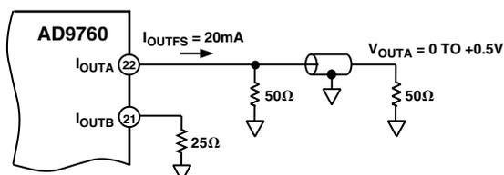
Figure 53. 0 V to +0.5 V Unbuffered Voltage Output
