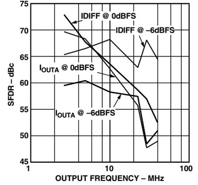
Figure 14. Differential vs. Single-Ended SFDR vs.  $f_{\text{OUT}}$  @ 100 MSPS
