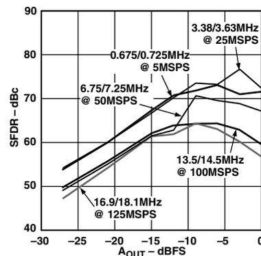
Figure 29. Dual-Tone SFDR vs.  $A_{OUT}$  @  $f_{OUT} = f_{CLOCK}/7$
