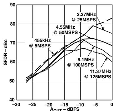
Figure 27. Single-Tone SFDR vs.  $A_{OUT}$  @  $f_{OUT} = f_{CLOCK}/11$
