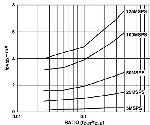
Figure 49.  $I_{DVDD}$  vs. Ratio @  $DVDD = 3$  V
