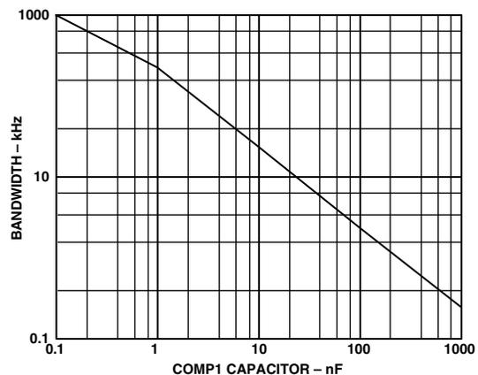
Figure 42. External COMP1 Capacitor vs.  $-3$  dB Bandwidth
