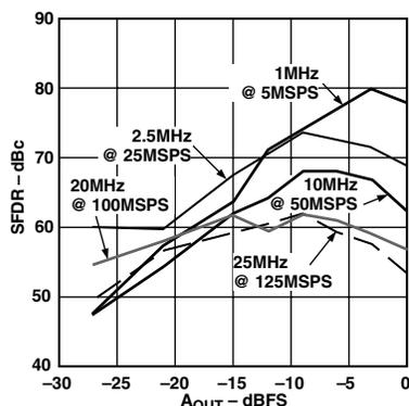
Figure 28. Single-Tone SFDR vs.  $A_{OUT}$  @  $f_{OUT} = f_{CLOCK}/5$
