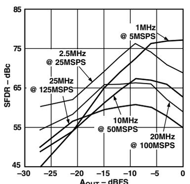
Figure 10. Single-Tone SFDR vs.  $A_{OUT}$  @  $f_{OUT} = f_{CLOCK}/5$
