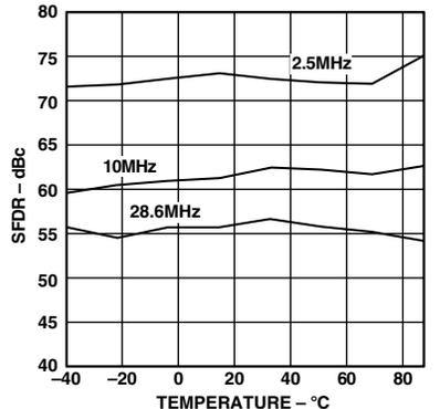
Figure 35. SFDR vs. Temperature
