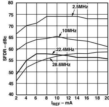
Figure 31. SFDR vs.  $f_{\text{OUT}}$  and  $I_{\text{OUTFS}}$
