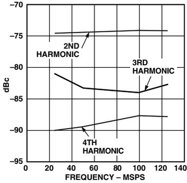
Figure 30. THD vs.  $f_{\text{CLOCK}}$
