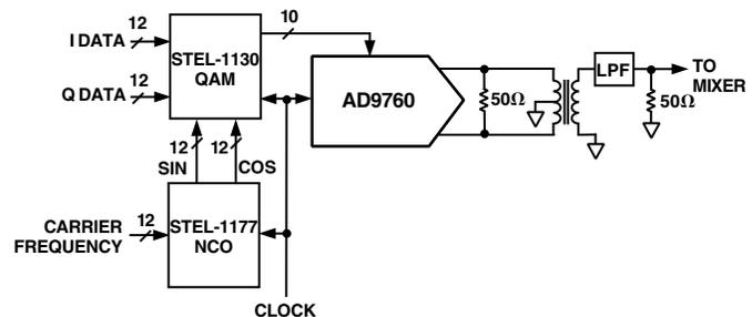
Figure 58. Digital QAM Architecture
