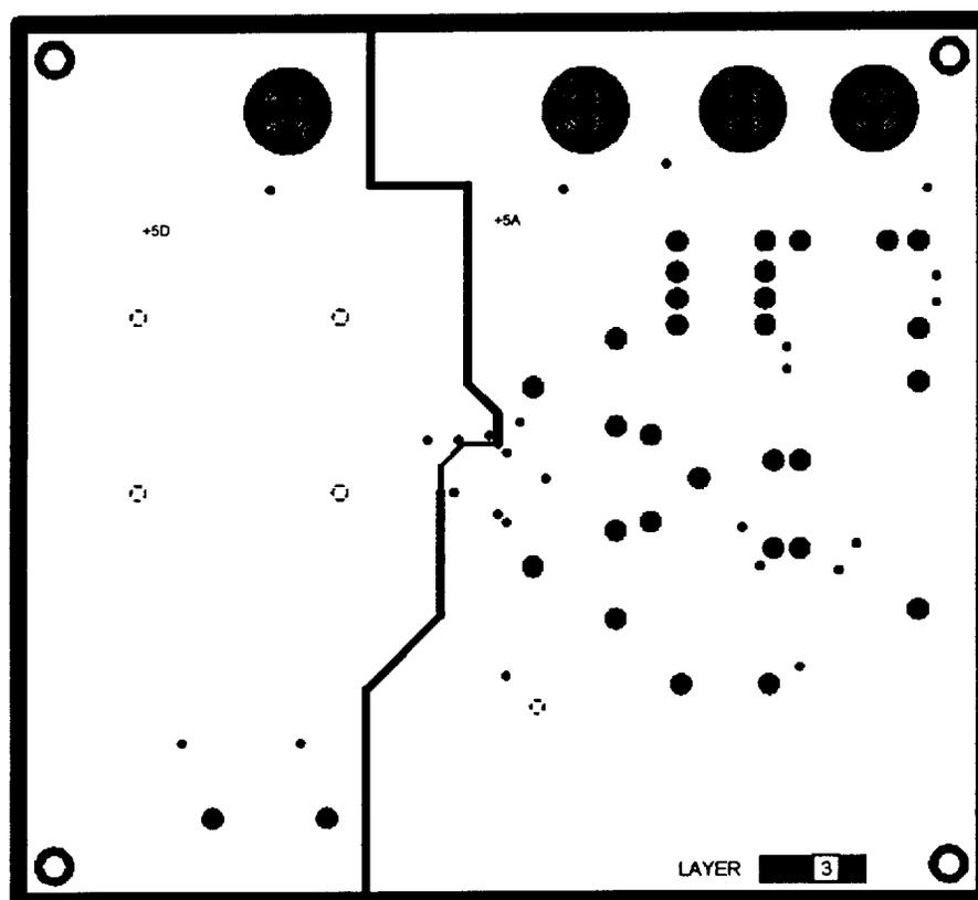
Figure 63. Power Plane PCB Layout (Layer 3)
