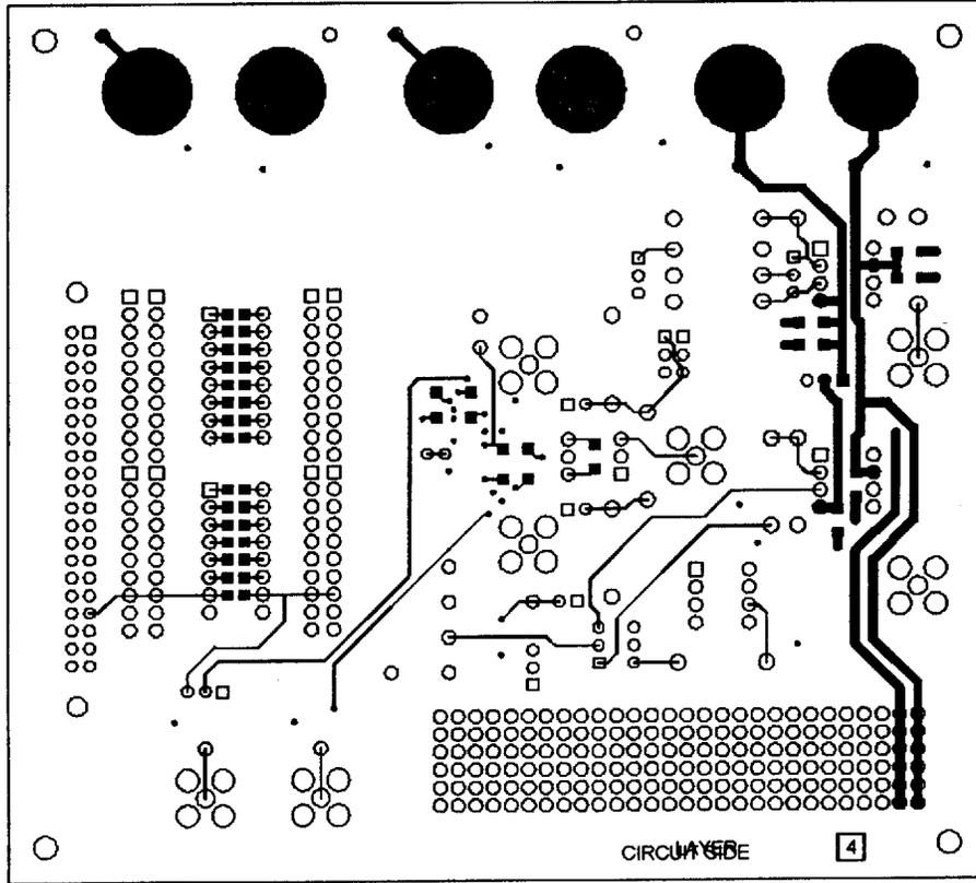
Figure 64. Solder Side PCB Layout (Layer 4)
