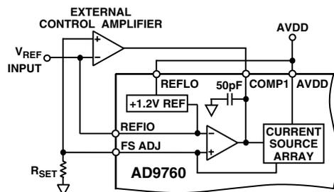
Figure 45. Configuring an External Reference Control Amplifier
