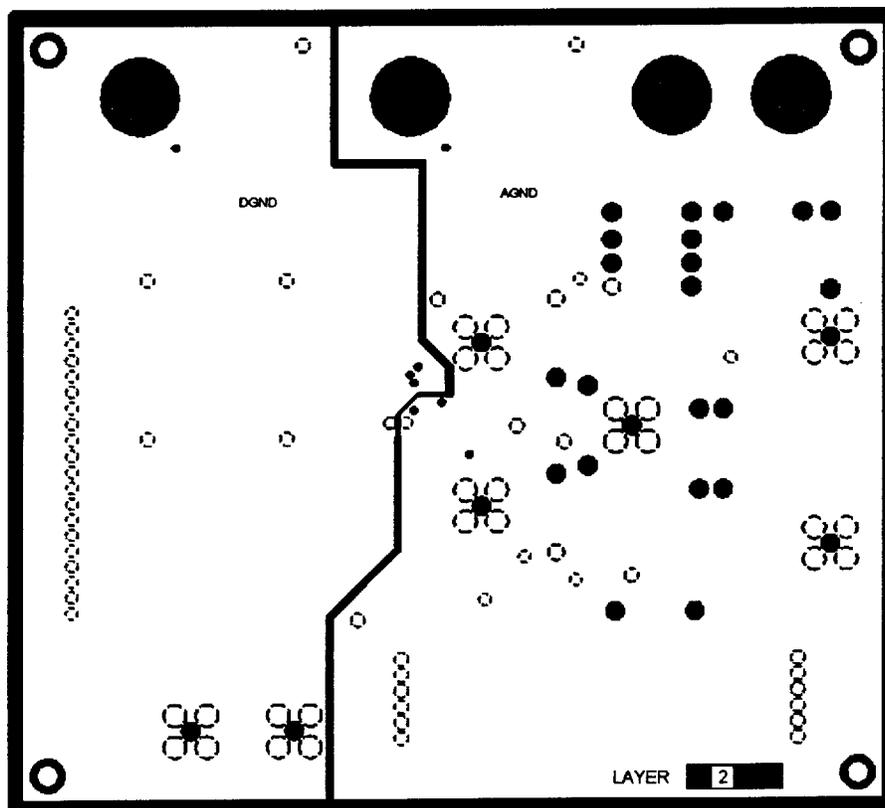
Figure 62. Ground Plane PCB Layout (Layer 2)
