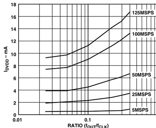
Figure 48.  $I_{DVDD}$  vs. Ratio @  $DVDD = 5$  V
