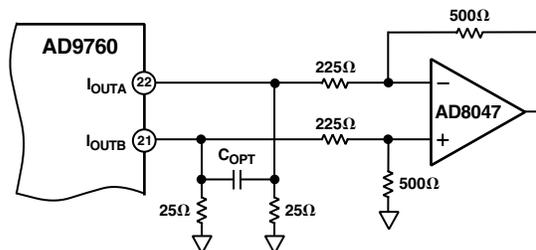
Figure 51. DC Differential Coupling Using an Op Amp
