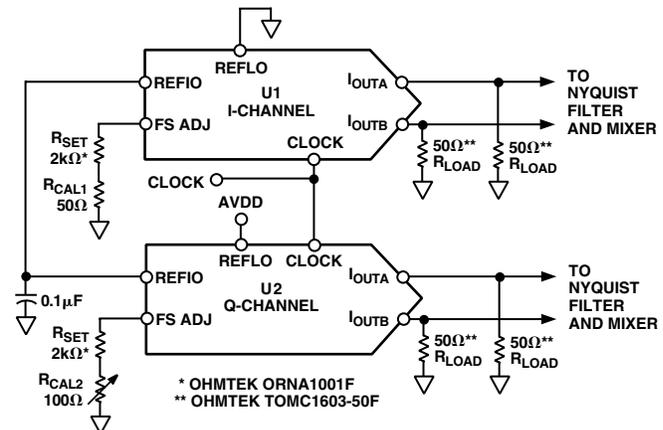
Figure 57. Baseband QAM Implementation Using Two AD9760s
