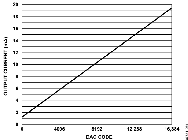
Figure 63. Gain Curve for FSC[9:0] = 512, DAC Offset = 1.228 mA
