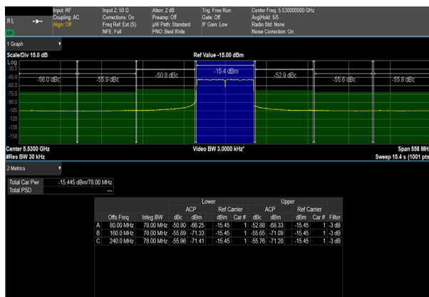
Figure 40. 80 MHz 802.11AC ACLR at 5530.0 MHz
