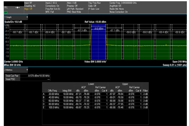
Figure 36. 20 MHz LTE Carrier ACLR at 3695.0 MHz
